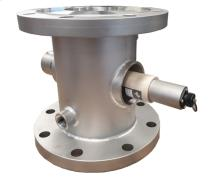
Turbidity Analyzer uses light in the near infrared (NIR) range from 730 to 970 nm. A precisely defined, constant light beam penetrates the liquid sulphur. Light scattered from particles in the medium is detected by eight hermetically-sealed silicon photo diodes at an angle of 11°. Simultaneously, the unscattered light is detected by a reference photo diode. If sulphur turbidity reaches an unacceptable level, the flow can be automatically recirculated or switched off.
