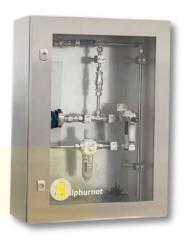
The Bubble Tube Level Measurement System is a self-contained, low-cost instrument designed for precise level indication in liquid sulphur melting tanks. This system operates by measuring liquid level through density and pressure, making it ideal for challenging environments like a sulphur melting tank.
