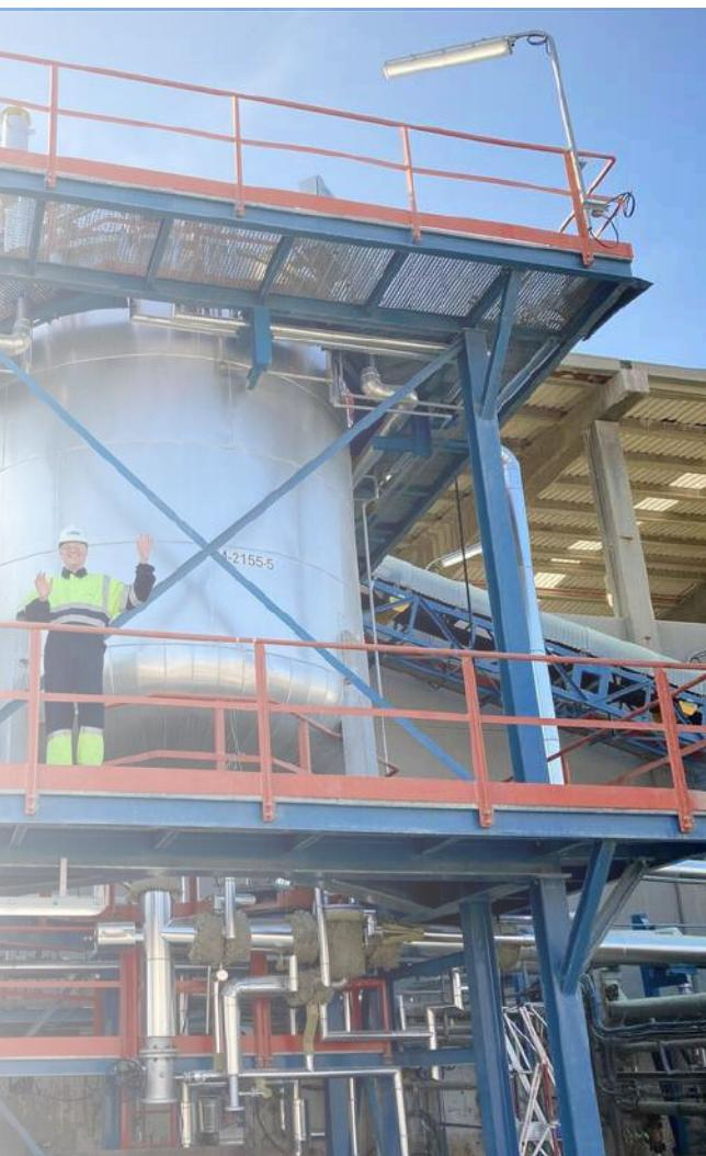
**Unmatched Efficiency:** Our tank can produce up to 70 metric tons of liquid sulphur per hour, making it one of the highest-capacity melters on the market.
